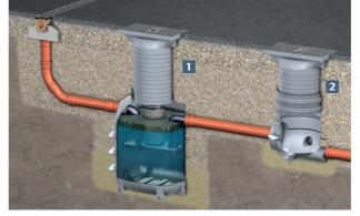
1 Coalisator-P light oil separator 2 Sampling shaft
