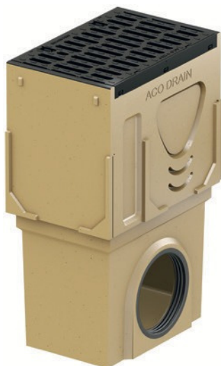
← ACO PointDrain E–F for classes E 600 – F 900, made of polymer concrete with cast iron grid, execution with lip labyrinth seal (LLD)
