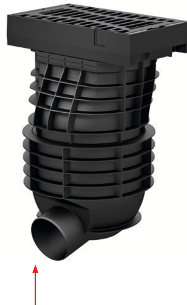
↑ ACO Combipoint PP road gullies for classes C 250 – D 400, made of plastic with cast iron top and grating, height-adjustable, rotatable, titable
