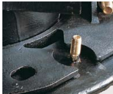
Detail of a Multitop HSD-2 bridge drain: adhesive flange and tension ring with seepage openings to clamp in the sealing membrane.
